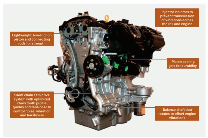
A meticulous engineering approach adds further performance and efficiency to the 2.0-liter EcoBoost engine. Twin independent variable camshaft timing (Ti-VCT) provides precise, variable timing control of both the intake and exhaust camshafts, which control the valve opening and closing events independently.
